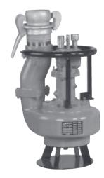
The Heidra 150V is a lightweight, compact 6" (150mm) hydraulic pump capable of passing large solids (up to 5"/125mm), stringy materials, and slurries with entrained gases. This pump is designed to pass through a standard 24" (610mm) manhole, making it ideal for sewer bypass applications.
